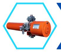
Scotch Yoke actuators are designed to operate ball, butterfly and plug valves requiring rotary quarter turn transition (on-off/modulating). Available as pneumatic and hydraulic, double-acting and spring return, also electro-hydraulic. A wide range of operating pressures, torque outputs and temperature ranges to suit an extensive variety of applications. Manual override, accessories and control panels are among available options.
