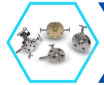
Monoflange valves in the Slim Line SB, SBB, DB, and DBB series feature inlet sizes from 1/2" to 4" (flanged) and threaded/flanged outlets. They are rated for ASME Class 150 lb to 2500 lb and API 3000 to 15000. The bonnet options include screwed and O.S&Y, bolted designs, with anti-tamper features and optional locking devices, suitable for cryogenic service.
